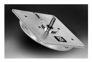
The Haydon™ 80000 Series stepper motor is designed for applications where accurate positioning, high torque and very thin packaging are desirable characteristics. This motor has a maximum diameter of 3.15-in (80 mm) and is less than 1/2-in (12.7 mm) thick.
