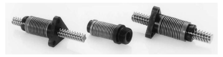
The ZBX assembly, through its unique transfer of loads, offers exceptional torque consistency and repeatability when traversing in either direction. The inherent damping qualities of the ZBX design make it ideally suited for vertical applications requiring noise or vibration control.
