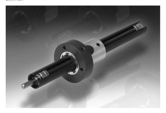
The ScrewRail consists of a precision rolled lead screw, supported by sealed bearings and contained within a concentric steel guide rail, driving an integrated nut/bushing. Because all the alignment requirements are achieved within the ScrewRail, support and positioning of the ScrewRail is much less critical than with traditional slide assemblies. Kerkote® TFE coating and self-lubricating nut/bushing materials ensure long life without maintenance.
