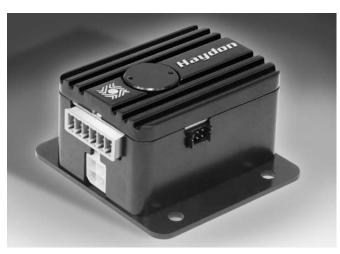
The Haydon™ DCM4826 IDEA Stepper Motor Drive is ideal for controlling both rotary stepper motors and stepper motor based linear actuator systems using a simple "pulse", "direction", and "enable" signal from a stepper motor control board. Input voltage to the drive is 12-48 VDC. The stepper motor drive can provide a load current of 2.6 A rms per phase. The PDE signals are optically isolated from the rest of the drive, providing the ability to reference a separate electrical ground.
