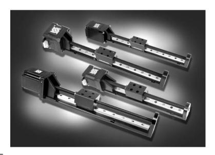
The **BGS™** Linear Rail combines many technologies into a single integrated linear motion platform. The system provides excellent load capability and is engineered for both normal and overhanging loads. High roll, pitch, and yaw moment loading capability allows the system to maintain tight accuracy and repeatability, even in applications requiring significant cantilevered loading.
