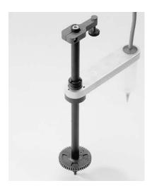
When mounted vertically, the ScrewRail can be used to simultaneously lift and rotate (Z-theta motion). With one motor driving the screw and a second rotating the rail, a compact, self-supporting pick and place mechanism can be created.
